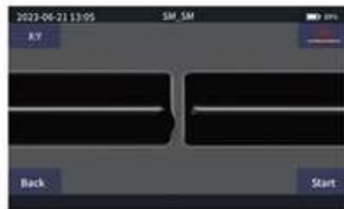
Uneven end face of optical fiber
